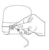
Place the AC Adapter cord around the strain relief.
